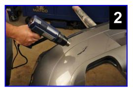
If bumper is distorted, it may be necessary to use a heat gun to restore the shape. This also helps dry the repair area.
