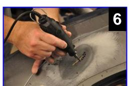
Drill 1/8" pinning holes around the perimeter of τne repair to create a mechanical bond.
