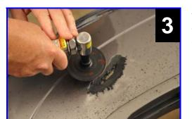
Taper, bevel and soften the edges of the repair with a 36 grit Trim-Kut Disc and an air grinder at slow speed to minimize melting / smearing of the plastic.
