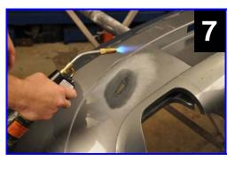
Flame treat the front and back sides of the repair with a propane torch. Simply pass the flame over the repair area
