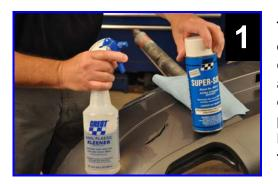
The front and back sides of the bumper must be cleaned before sanding to avoid grinding contaminants into the plastic. Clean first with **BPK-Vinyl Plastic Kleener**, then with ASX-Super Solv.
