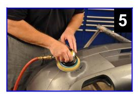
Sand the front and back sides with a DA and 80 grit sandpaper to remove any melted / smeared plastic and to finish shaping the repair.
