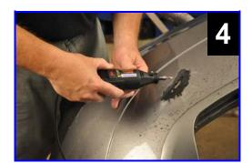
Enlarge the gap of the tear / crack to relieve binding / stress points and provide a passageway for the adhesive to flow.
