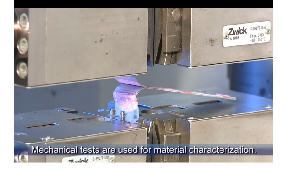
T-Peel and Lap Shear are typical experiments supporting adhesive development.
