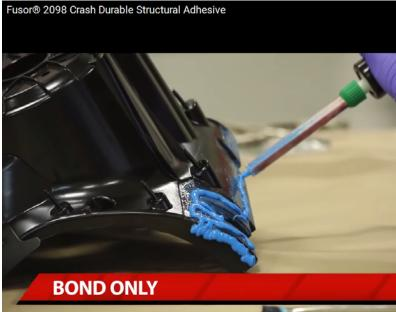
Dow Automotive -- Structural Bonding in modern lightweight vehicle design
